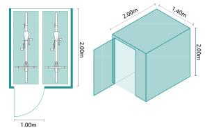
Figure 87: Secure cycle storage for two bicycles
