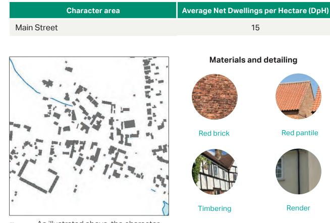
Figure 46: As illustrated above, the character area is organised across a fine urban grain street pattern radiating away from Main Street. Building sizes vary with both large (former agricultural buildings) and small (terraced and semi-detached properties) floorplates.
