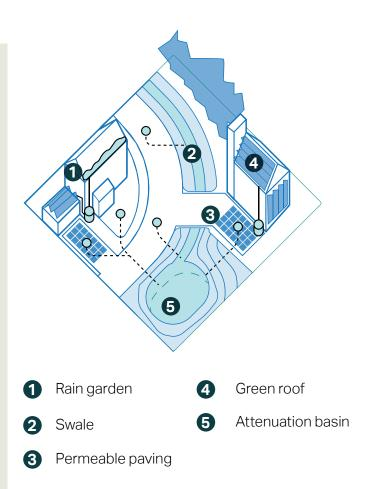
**Figure 97:** Diagram showing the best use of harvesting water systems rain garden, swales, permeable paving, green roofs
