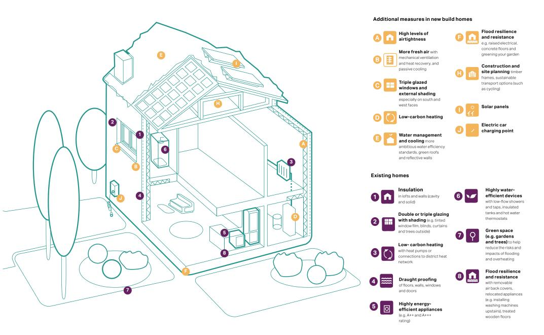
Figure 95: Cut-through diagram of an energy efficient home and its features.
