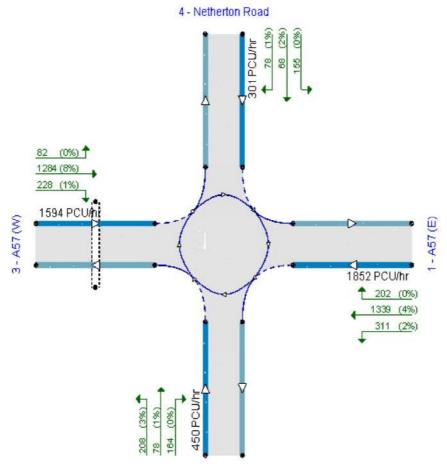
The junction diagram reflects the last run of Junctions.
