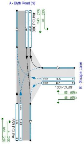
The junction diagram reflects the last run of Junctions.
