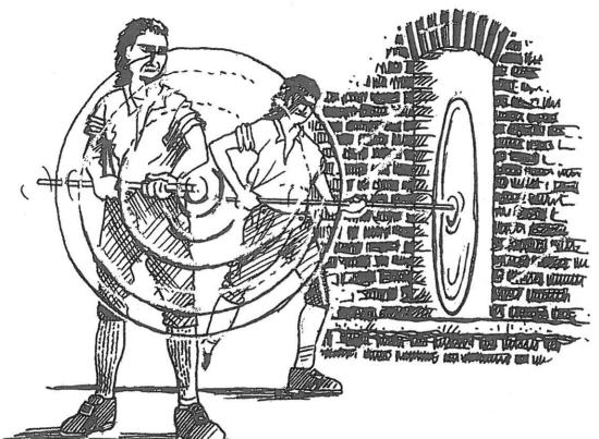
In the background, the bowl is being reheated and spun quickly. Centrifugal force has caused the bowl to flare out forming a flat disc or "table". This operation is known as "flashing".
