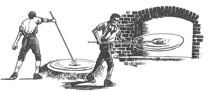
The completed 'table' is placed in an annealing oven which allows it to cool gradually.
