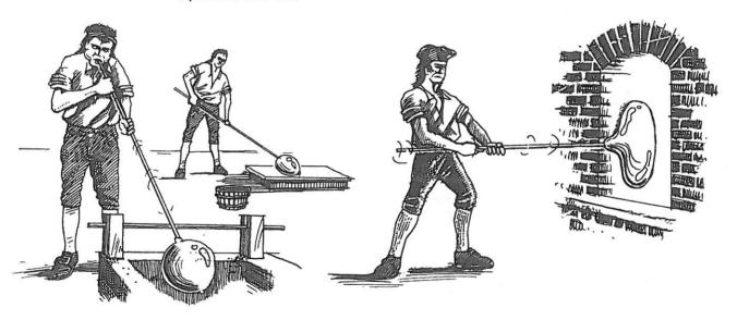
By a process combining blowing, reheating and rotating, a globe is formed at the end of the blowpipe.
