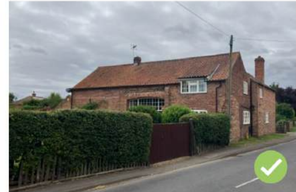
Figure 16: Clusters of old farm buildings with L-shaped arrangements are common, with main facades rotated at 90 degrees to the street, creating courtyards. Often gable ends extend right up to the pavement with no setbacks.
