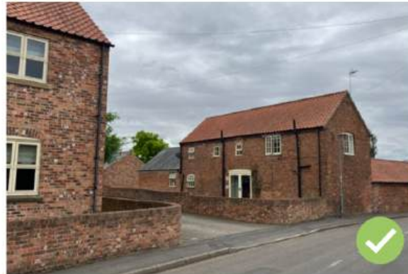
Figure 31: New development responds to and respects existing layouts, building lines and boundary treatments. On-plot parking is provided to the rear of dwellings.
