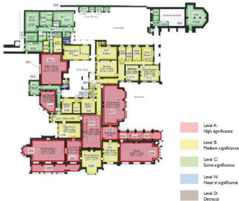
Plan to show levels of significance across the ground floor of a building (courtesy of The Prince’s Regeneration Trust, 2009)
